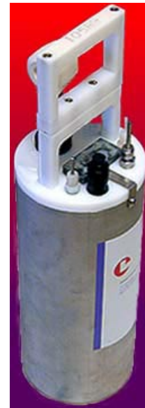
Coastal MacroQual (w/ CT, temp & pressure)
