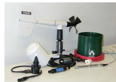
Optional Met Sensors (l to r) Radiation, External Temp Shield, Turbidity, External Pressure, Wind, RH, C-T, Rain Bucket
